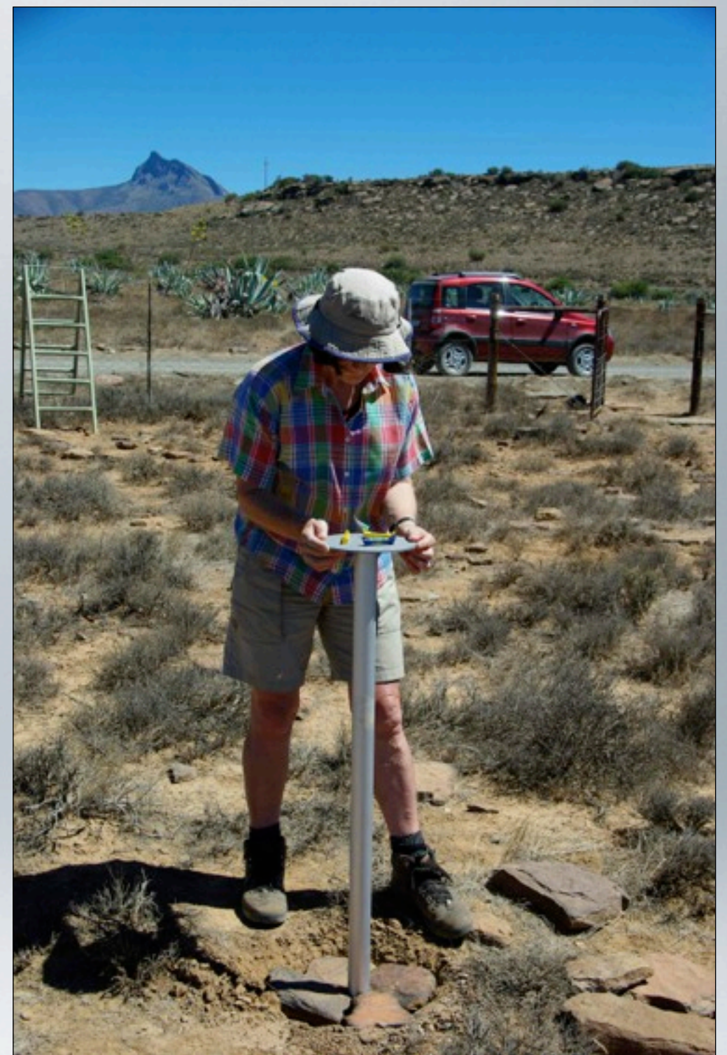
Installing the autographic rain gauge 25 January 2009
